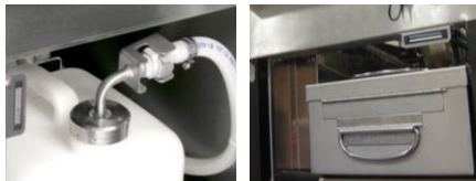
Oil replenished automatically from jug for multi-well (left) or reservoir for 1-well (right)
